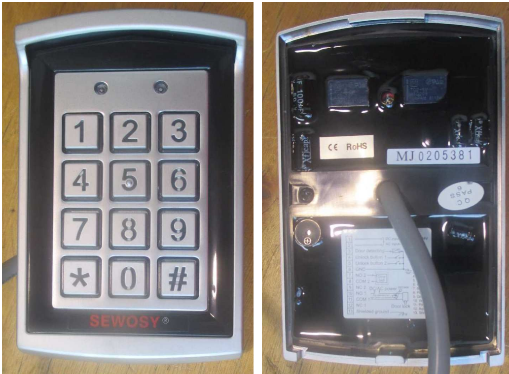
Keypad / proximity reader Type KRN 1000 before test
